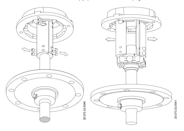
11. Removing the coupling leaves an open space that allows the extraction of the mechanical seal. Extract the lower shaft key so that the mechanical seal can slide out of the shaft. Loosen the set screws on the seal and remove it from the shaft.
