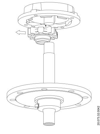
12. Insert the new mechanical seal in the shaft and slide it to a position that will allow the removal of the fixing tool and reinstalling the coupling.
