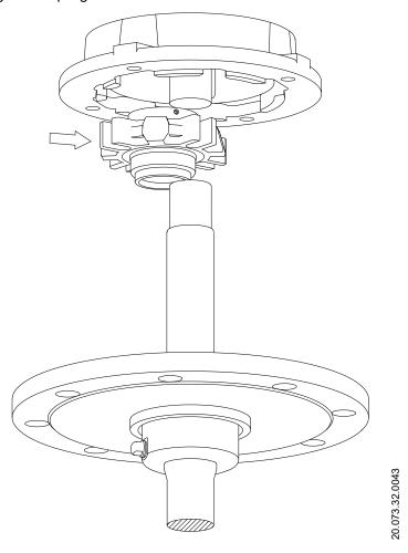
13. Insert the key in the lower shaft and reinstall the shaft coupling making sure the keys are aligned and correctly inserted in the coupling. The coupling faces should be parallel to each other before starting to tighten.
