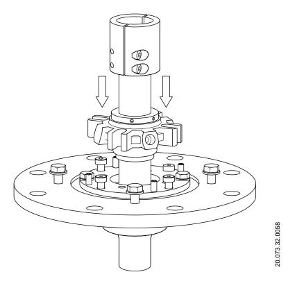
16. Tighten the 4 hex bolts but leave the set screws loose.
