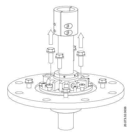
7. Slide the mechanical seal along the shaft away from the flange and tighten one of the set screws to fix the seal next to the shaft coupling and allow space for the following steps.
