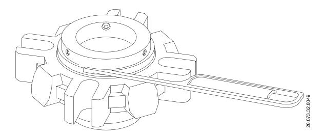
5. Tighten the shut-off nuts 2-3 turns at time and in a cross pattern to lower the shut-off flange until there is clear resistance in all 4 nuts.
