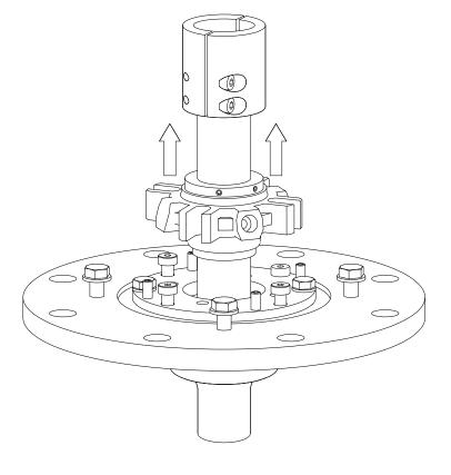
8. Place the shaft fixing tool in the position of the mechanical seal and insert the 2 screws in the fixing tool, screwing them in without tightening
